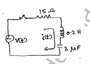
18. A voltage V (t) = 10 sin  $\omega$  t is applied to a series RLC circuit. At the resonance frequency of the circuit, the maximum voltage across the capacitor is found to be 500 V. Moreover, the bandwidth is known to be 400 rad/sec and the impedance at resonance is 100  $\Omega$ . Find the resonant frequency. Also find the values of L and C of the circuit.
