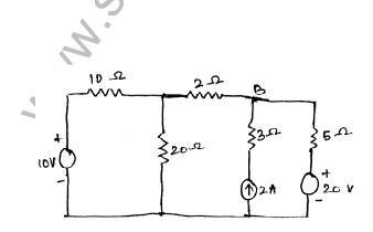
17. In the circuit shown in figure, determine the complete solution for the current, when the switch is closed at time t = 0. Applied voltage
