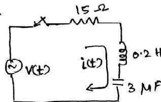
18. A voltage  $V(t) = 10 \sin \omega t$  is applied to a series RLC circuit. At the resonance frequency of the circuit, the maximum voltage across the capacitor is found to be 500 V. Moreover, the bandwidth is known to be 400 rad/sec and the impedance at resonance is 100  $\Omega$ . Find the resonant frequency. Also find the values of L and C of the circuit.
