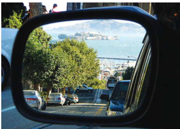
Used as rear view mirrors in automobiles since its field of view is wide.
