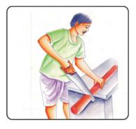
The wood is cut, when the saw is pushed and pulled through the wood.
