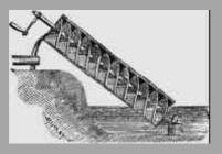
Such screws are still used in large machines for waste-water treatment and also in small machines which maintain blood circulation during heart surgery.
