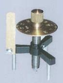
By placing its three legs on top of the piece of sphere, we can find the width of an arc. Using the screw in the middle, the maximum height can also be found.
