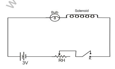
a) when the key is switched ON the bulb obtains maximum glow only after a shorter interval of time Which property of the solenoid is responsible for the delay?
